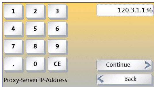
A keyboard will appear on the display in which you can enter the IP address.
