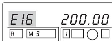
Diagnostic codes that begin with the letter C or E only occur during the reset process and usually pertain to the modem connection.
