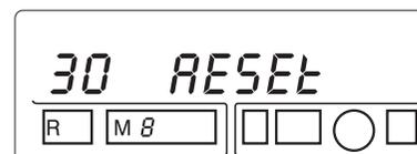
6. Within 30 seconds press the white 'TELESET' key again to confirm reset of the new amount. The display will count down from 30 to remind you. The process is then handled automatically. When complete the T-1000 will return to the ready mode.
